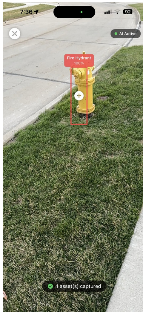
Figure 7.1 — AI Detection showing 'Fire Hydrant 100%' confidence with bounding box and capture button
