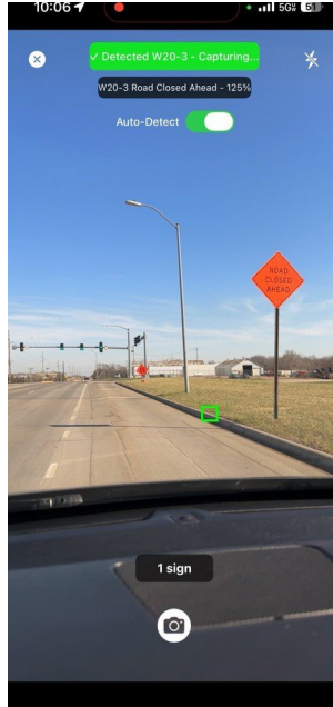
Figure 3.1 — Auto-Capture detecting a W20-3 sign at highway speed
